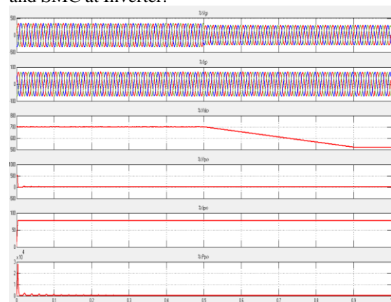
Fig. 12 Simulated performance for, (a) variations in the grid voltage, (b) variations the grid current, (c) adaptive DC voltage waveform as the voltages variations range upto 20% at CPI, (d),(e),(f) shows the voltage ,current and power waveforms of PV panel
