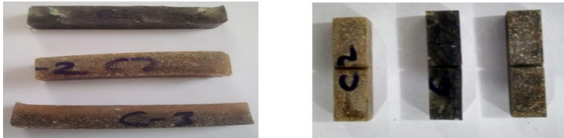
Fig: (3.4): Cutting specimens for Izod & Charpy-V Impact test specimens
