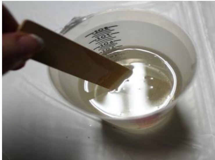
Fig: 2.4. Polyester resin in stirring process
