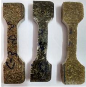
Fig (3.1).D: Tensile testing Specimens Before testing
