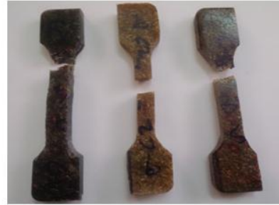
Fig (3.1).E: Tensile testing specimens after testing
