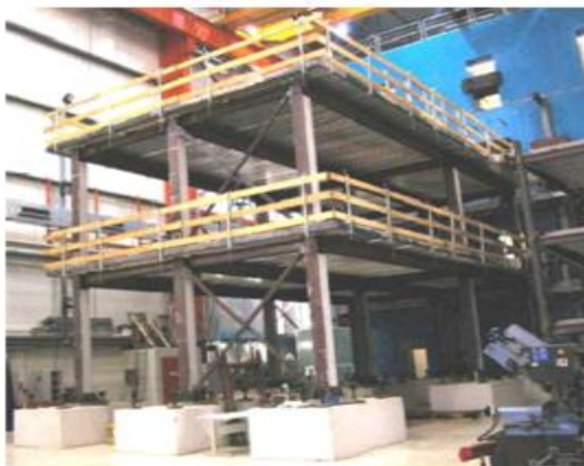
Fig. 5. Front-side picture of the test structure
