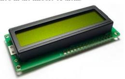
The internal surface of the glass plates are covered with straightforward cathodes which characterize the character, images or examples to be shown polymeric layers are available in the middle of the terminals and the fluid precious stone, which makes the fluid gem particles to keep up a characterized introduction point. One every polarizers are glued outside the two glass boards. These polarizers would pivot
