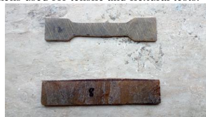
Fig 3. Prepared specimens for tensile and flexural tests
