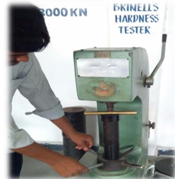
Fig 12: Testing hardness by Brinell hardness tester.
