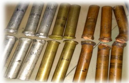
Fig 15: Tested samples under tension
