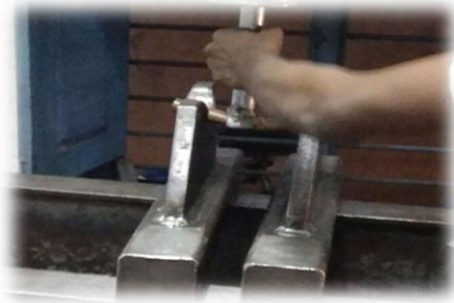
Fig 13: Testing the weld strength by applying hydraulic load
