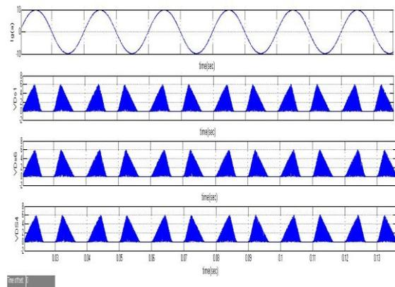
Figure 21: Drain to source voltage of different switches S1, S6 and S4
