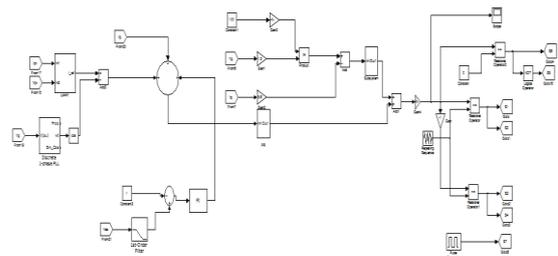
Figure 16: control diagram with PI controller
