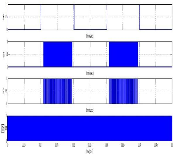
Figure 19: Gates pulses of switches S6, S1, S3 and S7
