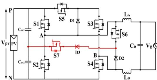
Fig 3 proposed transformer less grid-connected PV inverter structure
