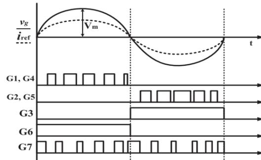
Fig 4 Gate drive signals of the proposed topology
