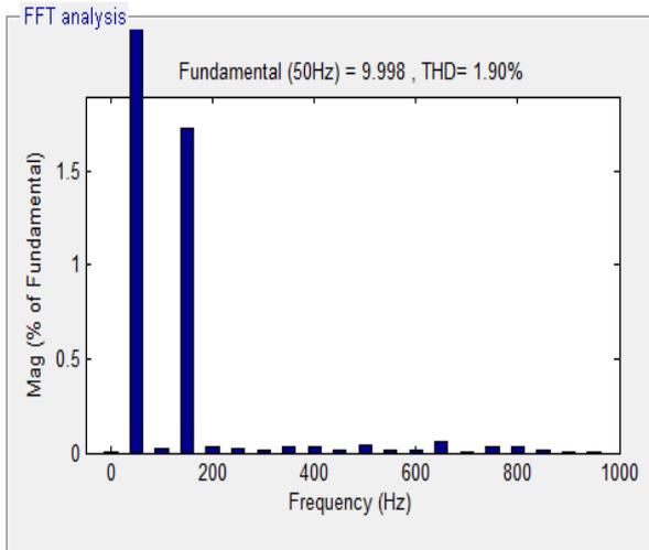
Figure 17: Total harmonic distortion of output current Using PI controller
