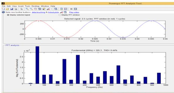
FiFig 23 Total harmonic distortion of output voltage with Fuzzy controller
