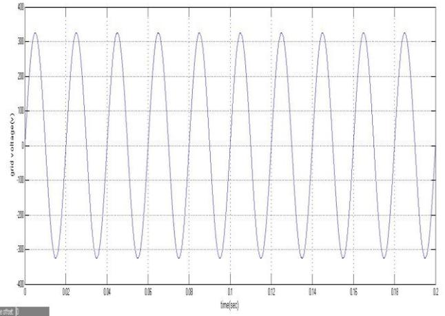
Figure 25 Grid voltage
