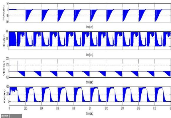
Fig.7.24: Voltages and currents of Switch S2 and S3
