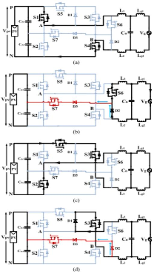
Fig. 5. Operating principle of the proposed topology: (a) Active and (b) freewheeling modes in the positive half cycle of the grid current, (c) active and (d) freewheeling modes in the negative half cycle of the grid current.
