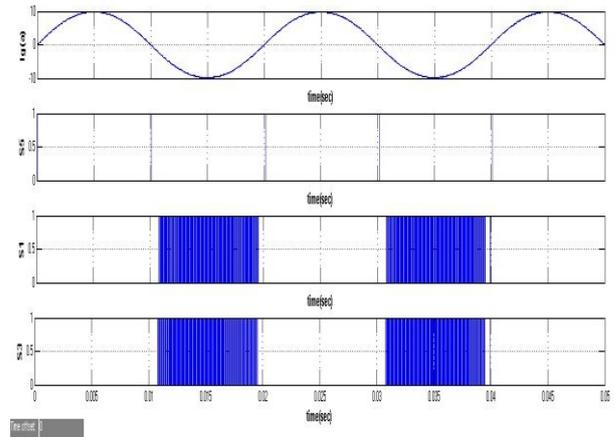
Figure 20: Grid current(Ig) and gate pulses for switches S6, S1 and S3
