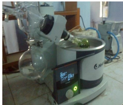
Figure 7: Rotary evaporator used for removal of the solvents in crude extract
