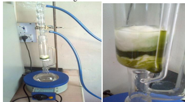
Figure 5: starts extraction using soxhlet apparatus, phytochemicals dissolves in solvent (left to right)
