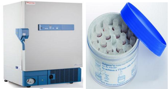
Figure 2: -80°C freezer, Mr.Forsty freezing container
