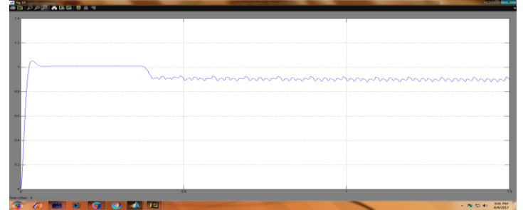
Fig.18 DC link voltage
