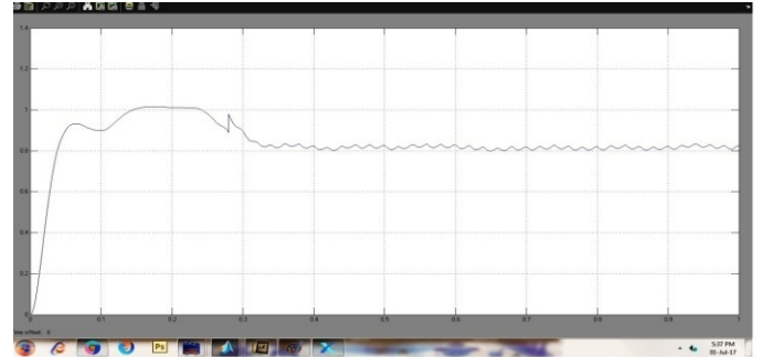
Fig.37 DC link voltage.
