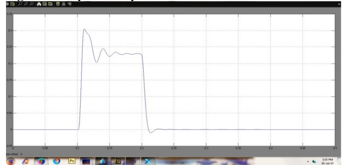
Fig.37 DC link voltage.
