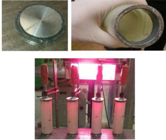
(b) Tubes clamped and under heating lamp for the pre-cure of the adhesive.
