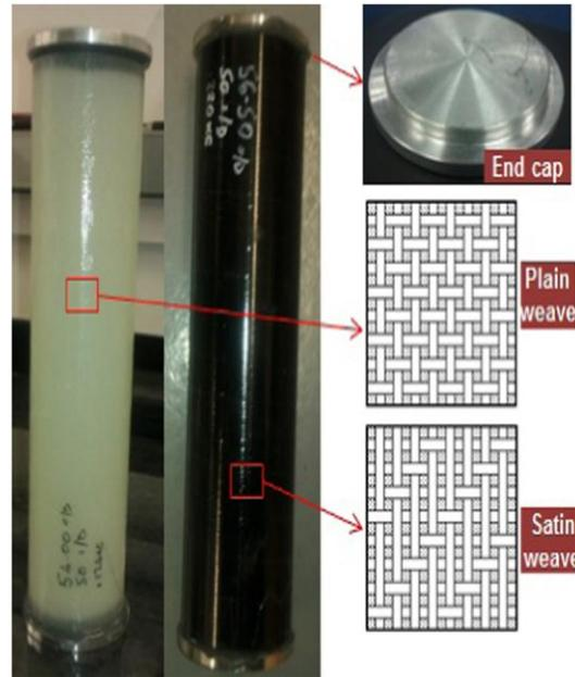
Fig. 4 Illustration of specimens with fitted end caps prior to testing
