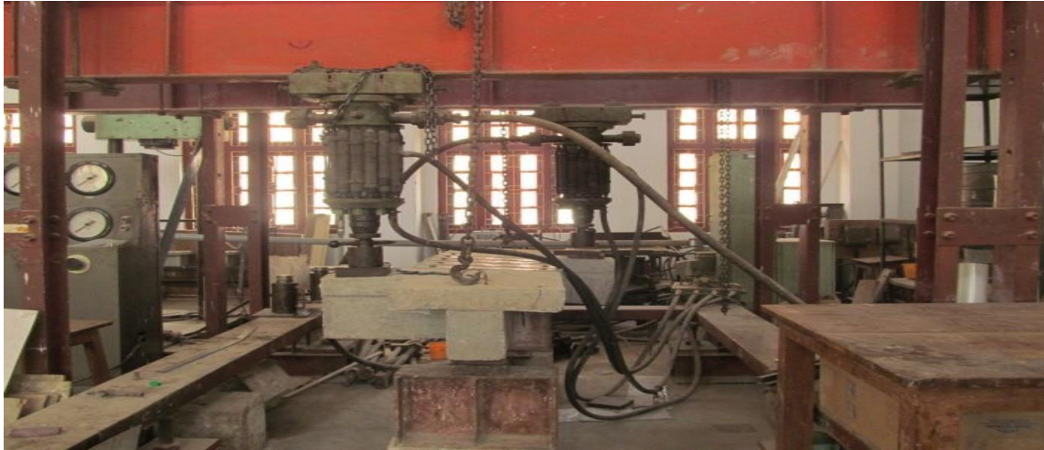
Figure-2 S.F and B.M Diagram for 2-Point Loading and Loading Setup
