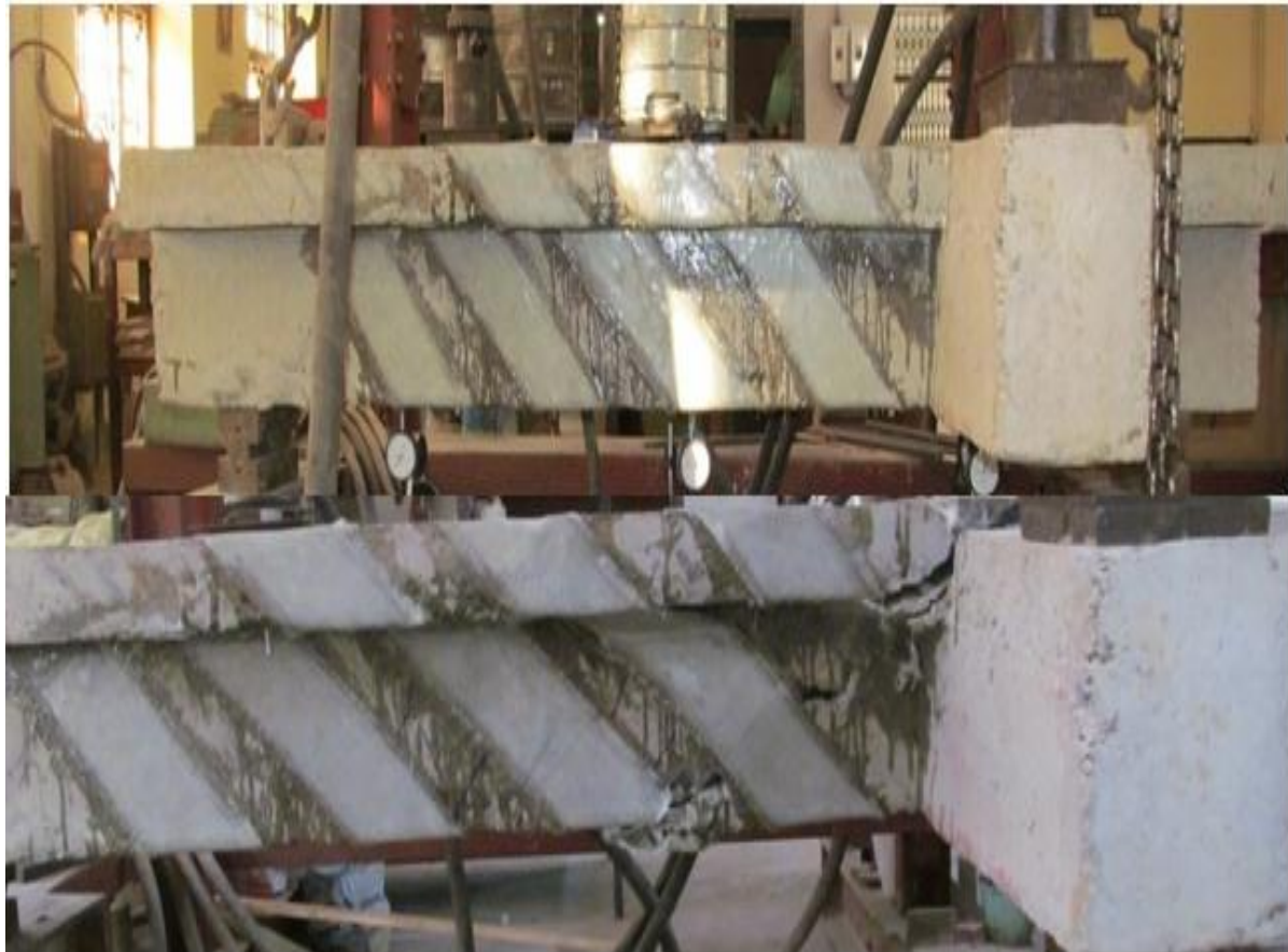
Figure-4 Beams retrofitted with GFRP oriented at 45°
