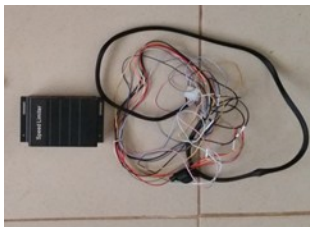
Figure 9. Road Speed Limiter Device and Power Cable
