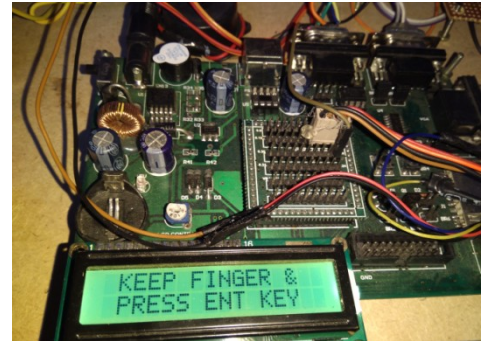
Fig:5: first we have place our finger and has to press enter key
