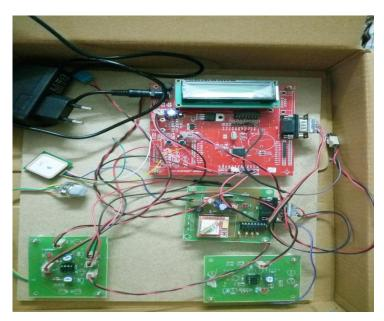
It consists of six main modules power supply, lcd display, sensors, gps receiver, microcontroller and gsm.
