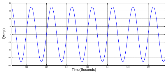
Fig.14 Output waveform of the inductive filtering TCR and TSC method
