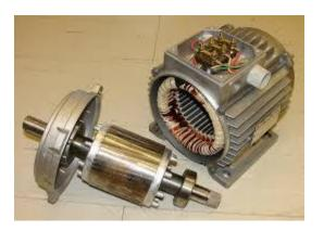
The construction of single phase induction motor is almost similar to the squirrel cage three phase motor except that in case of asynchronous motor the stator have two windings instead of one as compare to the single stator winding in three phase induction motor.
