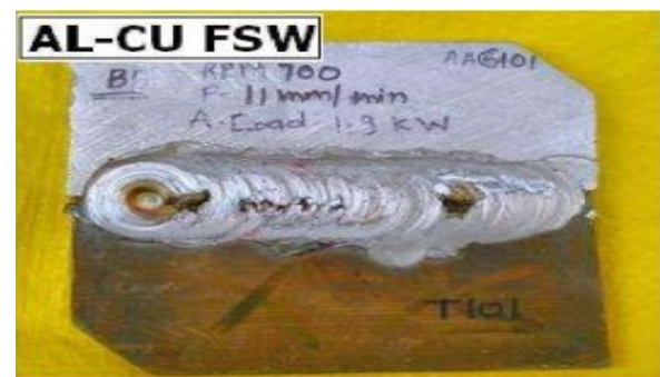
Figure:2 Photograph of Dissimilar joint Copper and Aluminium AA6101
