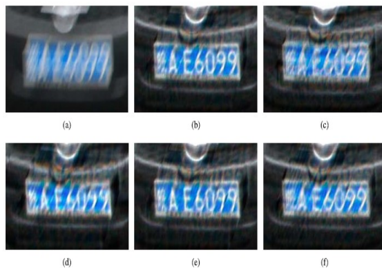
Fig 1 (a) blurred image (b) ( \theta = 66.67^\circ, l = 29.87 ) (c) ( \theta = 66.67^\circ, l = 24.87 ) (d) ( \theta = 66.67^\circ, l = 34.87 ) (e) ( \theta = 61.67^\circ, l = 29.87 ) (f) ( \theta = 71.67^\circ, l = 29.87 )
