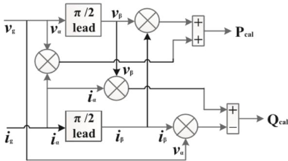
Fig. 11. OSG based power calculation.
