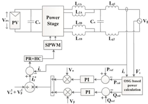
Fig. 10. Control diagram of the proposed topology.
