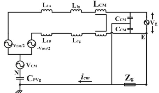
Fig. 8. Simplified CM model at switching frequency for positive half cycle.
