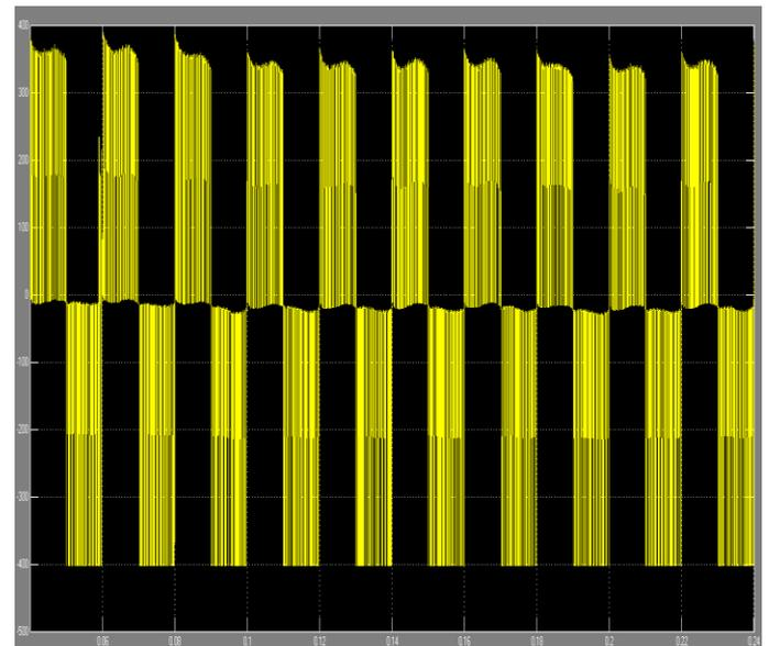
Fig.14 Inverter 3-level output voltage
