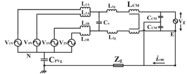
Fig. 7. Equivalent CM model of the proposed topology.
