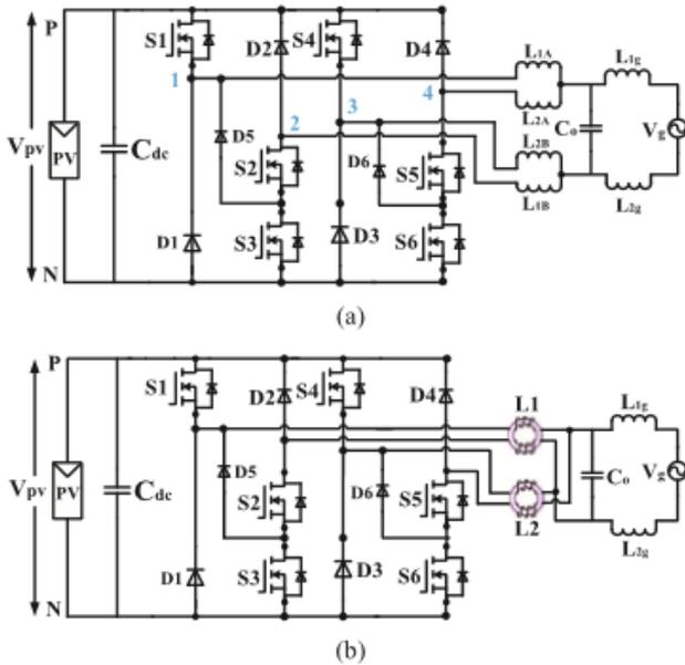
Fig. 4. (a) Circuit structure of the proposed transformerless topology for grid-tied PV system (b) circuit structure with coupled inductor.
