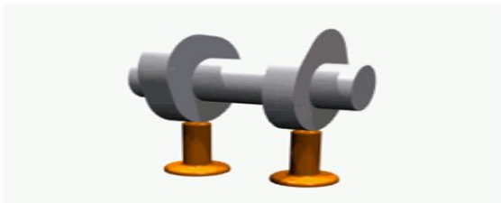
Fig 4 Cam shaft working
