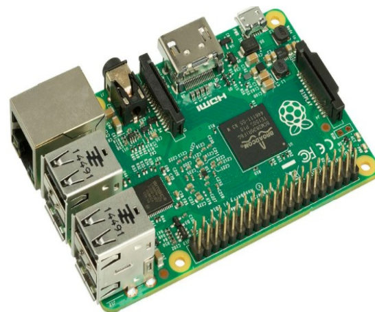
Fig 4 The Model B boards incorporate four USB ports for connecting peripherals.
