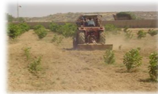
Fig 1 (e) Rough Leveling with Rear Blade Fig 1 (f) Rough Leveling with Rear Blade
