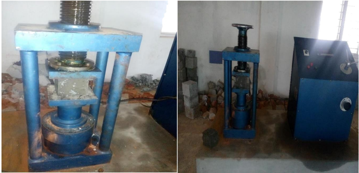
Fig Compressive Strength Test of (3,7,21,28 days) Cubes using CTM
