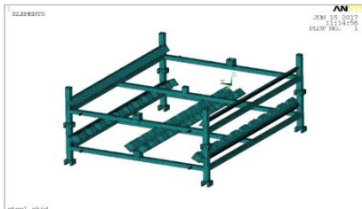
Fig. 4.3. Finite element model of the skid
