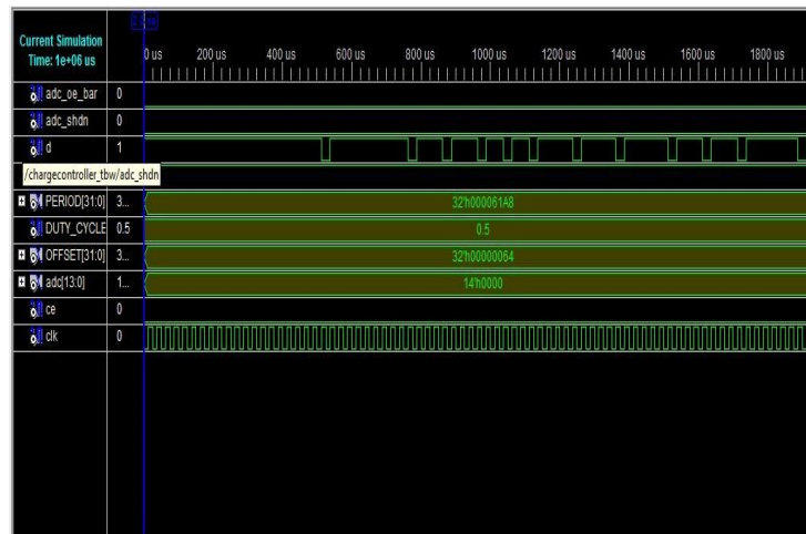
Fig.14. Firing pulses to BDC in boost mode
