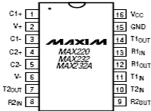
Fig:4. Pin diagram of MAX232 IC
