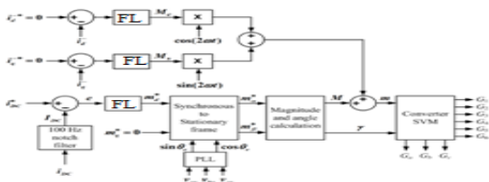
Fig. 9. Block diagram of the proposed control scheme to inject balanced three-phase grid currents under unbalanced grid voltage conditions.
