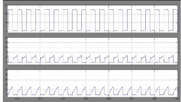
Fig.9. Simulation waveform of diode voltage (Vds), diode Current (Id4), diode Current (id3).
