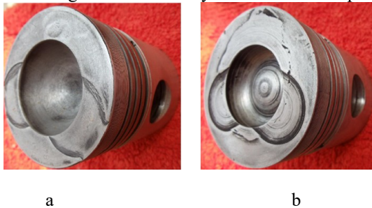
Fig.3 (a) Hemi Spherical Open Combustion Chamber Fig. 3 (b) Re-entrant Open Combustion Chamber
