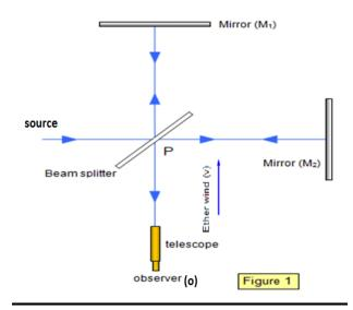
Light from a source falls on a beam splitter P, a partially coated mirror that partly reflects; partly transmit light, as is shown in Fig1. The reflected beam travels back and forth in one arm of interferometer  $PM_1$ , the transmitted beam in other  $PM_2$
