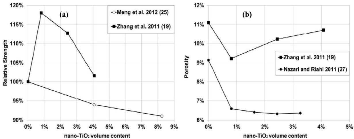
**Fig. 5.** (a) Nano-TiO<sub>2</sub> volume content x relative compressive strength [19,25]; (b) Nano-TiO<sub>2</sub> packing effect [19,27].
