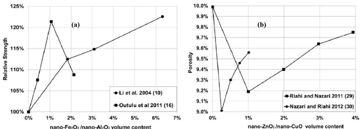
**Fig. 6.** (a) Nano-Fe<sub>2</sub>O<sub>3</sub>/Al<sub>2</sub>O<sub>3</sub> volume content x relative compressive strength [10,16]; (b) Nano-ZnO<sub>2</sub>/CuO Packing effect [29,30].
