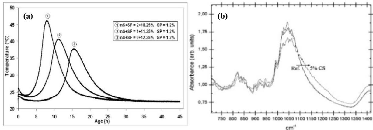
**Fig. 4.** Adiabatic Calorimetry of cement pastes with 0, 1, and 2% of nano-SiO<sub>2</sub>, reprinted with permission from L. Senff, D. Hotza, W.L. Repette, V. Ferreira and J.A. Labrincha // *Advances in Applied Ceramics* **109** (2010) 104, (c) 2010 Maney.
