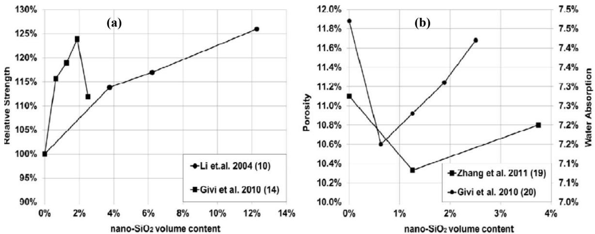
Fig. 2. (a) Nano-SiO<sub>2</sub> volume content x relative compressive strength [10,14]; (b) Nano-SiO<sub>2</sub> packing effect [19,20].
