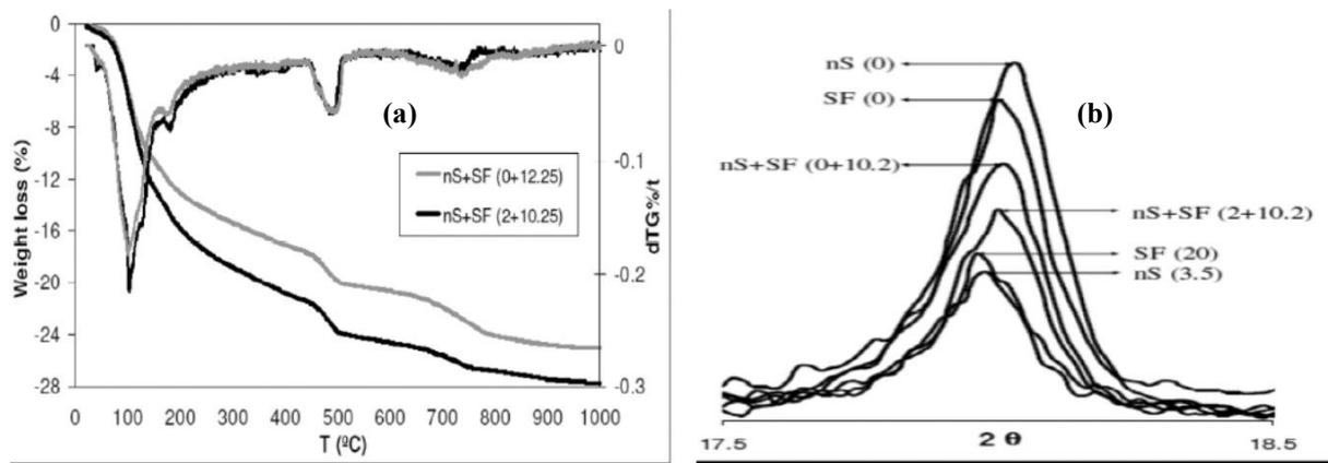
**Fig. 3.** (a) Thermogravimetric analysis results for cement pastes containing nano-SiO<sub>2</sub>, (b) DRX of Ca(OH)<sub>2</sub> peaks, reprinted with permission from L. Senff, D. Hotza, W.L. Repette, V. Ferreira and J.A. Labrincha // *Advances in Applied Ceramics* **109** (2010) 104, (c) 2010 Maney.
