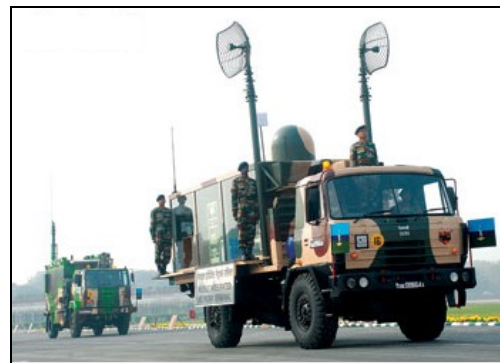
Figure 1.1: Mobile Radio Engineered Network Terminal
