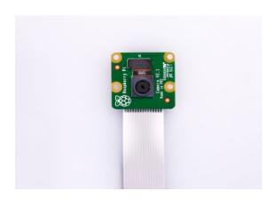
The Raspberry Pi Camera Module v2 is a high quality 8 megapixel Sony IMX219 image sensor custom designed add-on board for Raspberry Pi, featuring a fixed focus lens. It's capable of 3280 x 2464 pixel static images, and also supports 1080p30, 720p60 and 640x480p60/90 video. It attaches to Pi by way of one of the small sockets on the board upper surface and uses the dedicated CSi interface, designed especially for interfacing to cameras.
