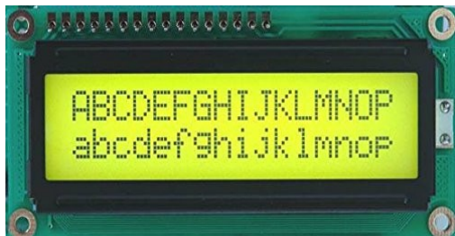
Figure 6 : liquid crystal display
