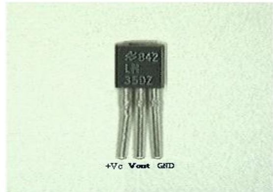
Fig.6: Temperature sensor- The LM35
