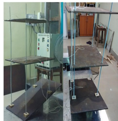
Figure 3.6: Experimental Model for 15^\circ slope
