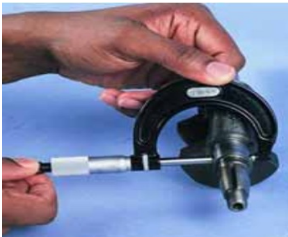
Figure.3 A micrometer is required to accurately measure bearing surface diameter on a crankshaft
