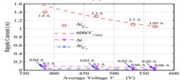
Figure 14. DC-bus current  $i$  and capacitor currents  $i_{C+}$  and  $i_{C-}$  over a wide range of  $V_{ave}$ .
