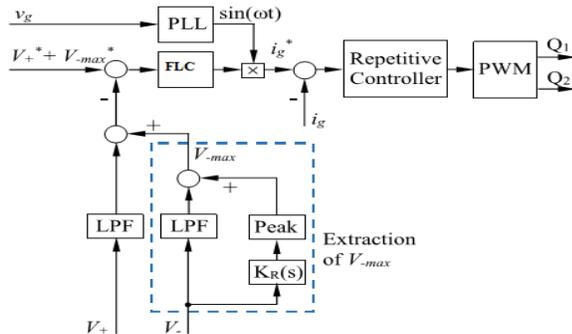
Figure 4. Controller for the rectification leg.
