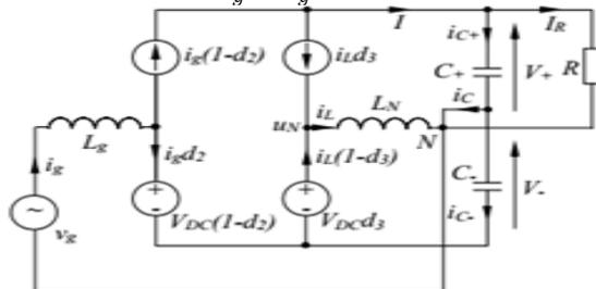
Figure 2. The average circuit model of the rectifier shown in Figure 1.
