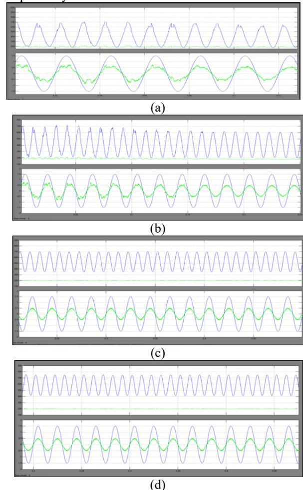
Figure 9. Grid voltage  $v_g$ , grid current  $i_g$  and DC voltages  $V_+$  and  $V_-$  with  $V_+^* = 200$  V: (a) when  $V_-^*_{max} = 600$  V, (b) when  $V_-^*_{max} = 650$  V, (c) when  $V_-^*_{max} = 700$  V, (d) when  $V_-^*_{max} = 750$  V.
