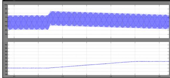
Figure 16. Transient response when the reference of the voltage  $V_+$  was changed from 200 V to 300 V.
