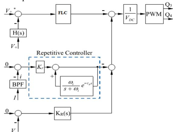
Figure 3. Controller for the neutral leg
