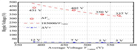
Figure 10. Voltage ripples of  $V_{+}$  and  $V_{-}$  over a wide range of  $V_{ave}$ .
