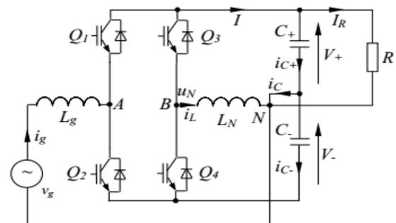
Figure 1. The single-phase rectifier under investigation.
