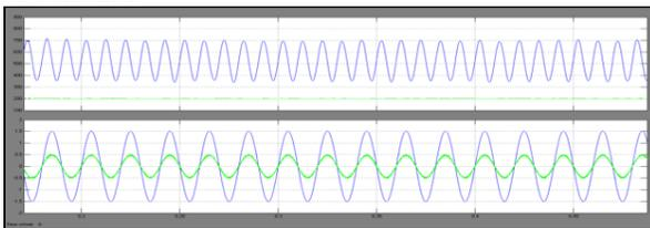
Figure 12. Deteriorated system performance when the controller that removes fundamental component from  $i_{C-}$  was disabled ( $V_{-max} = 700$  V)
