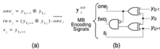
Fig.1 (a) Boolean equations and (b) gate level representation for the execution of the MB encoding signals.
