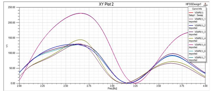
Figure 3. VSWR curves for various substrate materials.
