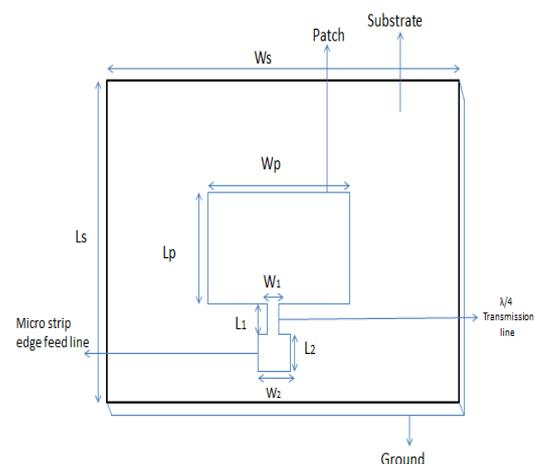
Figure 1. Graphite Based Rectangular Microstrip patch antenna.
