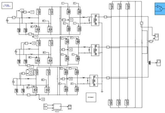
**Fig 7 simulation circuit of proposed converter**
