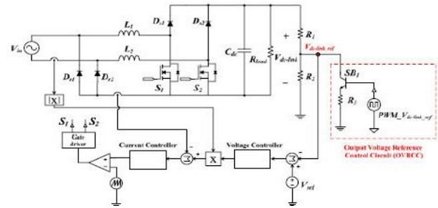
Fig.4 Schematic of PFC rectifier with the control circuit of output voltage reference
