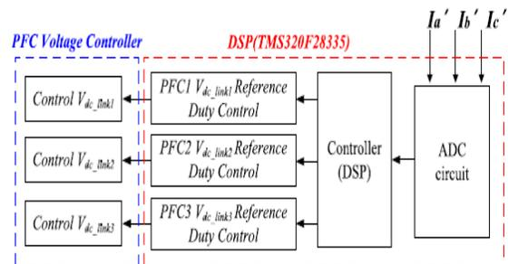
**Fig.6 Control strategy of the proposed current balancing algorithm using analog and DSP controllers**
