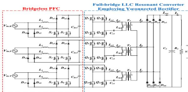
Fig.1. Circuit diagram of the proposed isolated ac-dc high-frequency-link Power-conversion system
