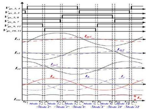
Fig.3. waveforms of the proposed converter
