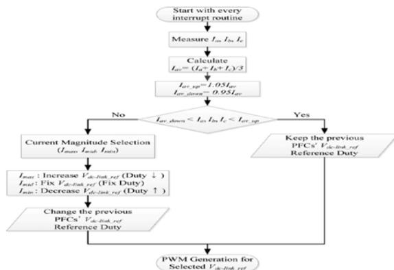
**Fig.5. Proposed current balancing algorithm**
