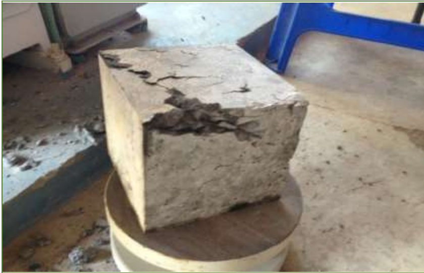
Figure 5. Represents the Concrete specimen of grade M60 with 5% fly ash and 1.0% SP430
