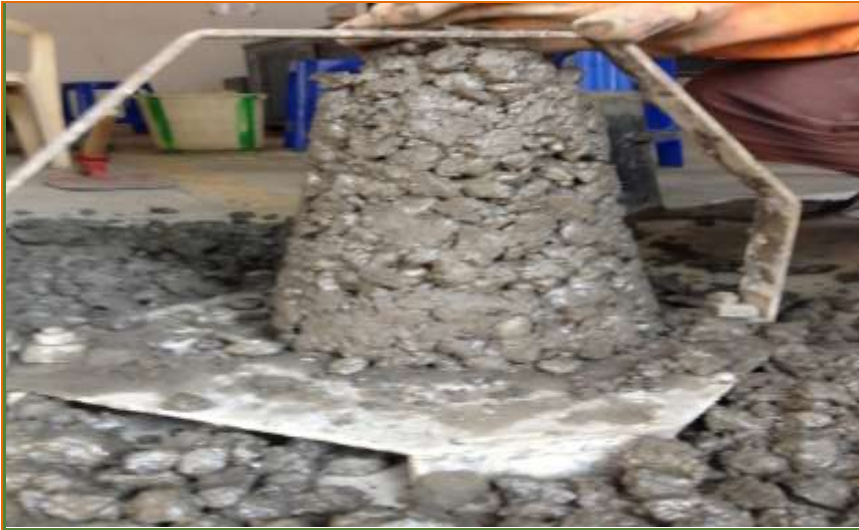
Figure 3 . Represents the Slump cone for Trial mix containing 0% fly ash and 1.0% SP 430
