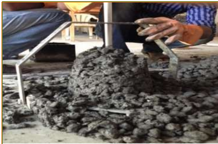
Figure.4. Represents the Slump cone of trial mix i.e. mix with 7.0% fly ash and 1% SP430
