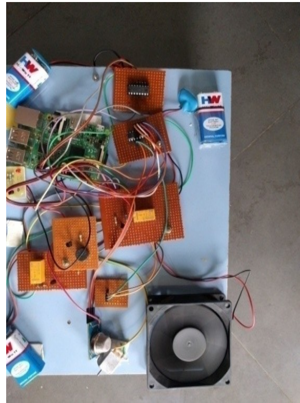
When temperature greater than 25 ° C fans is ON
