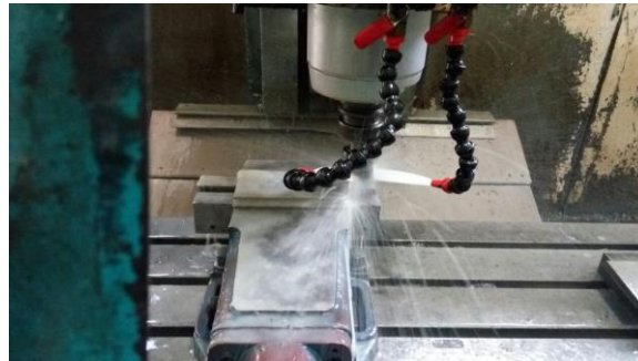
Machining of work piece by applying parameters – Spindle Speed 1000rpm, Feed Rate – 80mm/min and Depth of Cut – 0.5mm, Tungsten Carbide Tool
