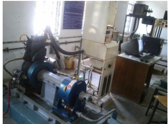
Figure – 3.10 A VCR Engine connected with computer system
