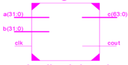
FIG 5. RTL SCHEMATIC OF DUAL MODIFIED ADAPTIVE MULTIPLIER.
