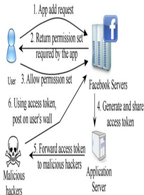
Fig: Steps involved in hackers using malicious applications to get access tokens to post malicious content on victims' walls.
