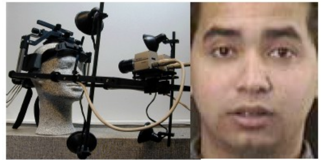
Fig. 4: Mounted-camera device and an example of an input frame
