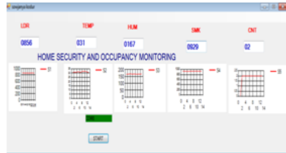
Fig10 Real-time Graphical representation of different types of sensing information on the IOT system when log in as local
